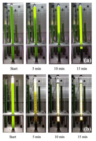
Fig. 3. Pilot-scale of microalga coagulation in 4 L column photobioreactors during 15 min reaction times: BBM medium (a) and DWW (b).
